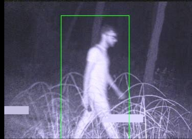
(Top) TrailGuard AI image of Piyush at night, transmitted from a small LoRa-GSM gateway, then on to the Internet, and ultimately received by designated parties as email alerts within 3 minutes.
